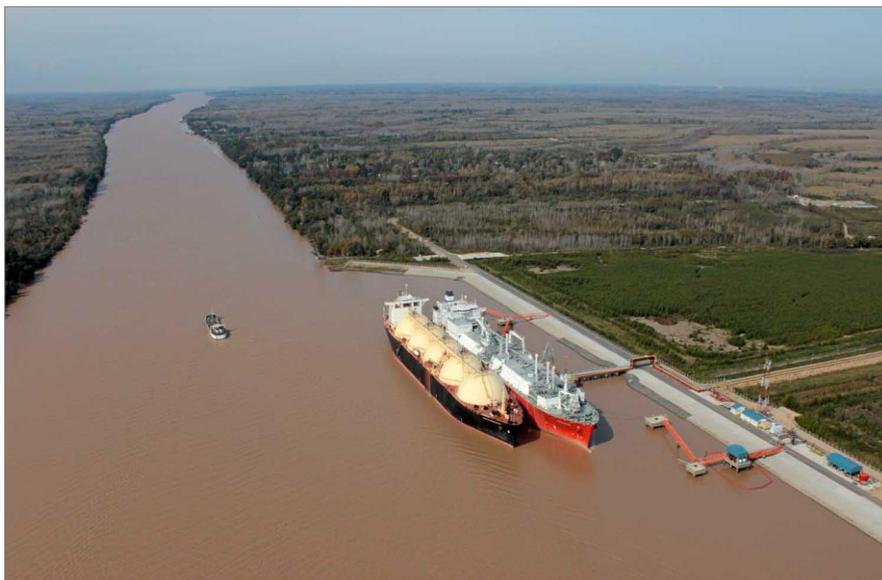
**Figure 7. LNG Carrier discharging to FRSU in Escobar LNG Terminal**
